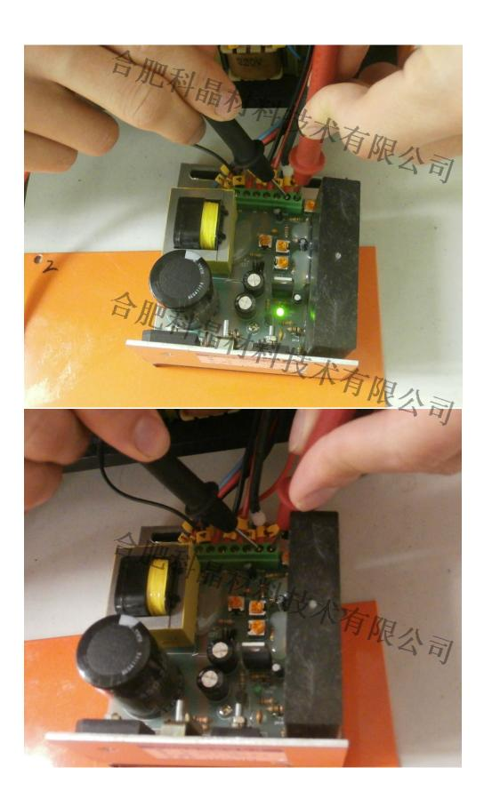
6. At last please check #3 and #4: the result should be 0V when the speed is minimum, then the result will increase if you increase the rotate speed
